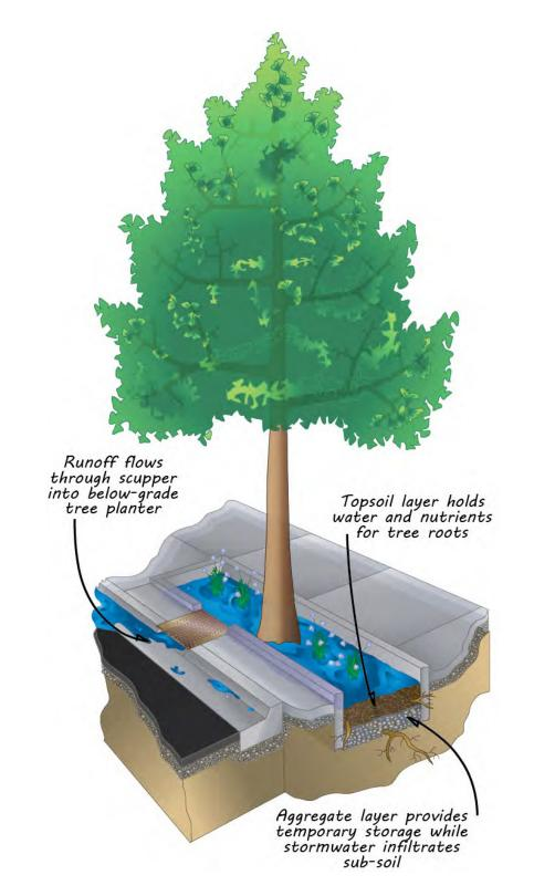
**Above:** Stormwater tree pits are designed to collect runoff from streets, parking lots, and other impervious areas. Stormwater is directed into scuppers that flow into below-grade planters that then allow stormwater to infiltrate soils to supplement irrigation.
