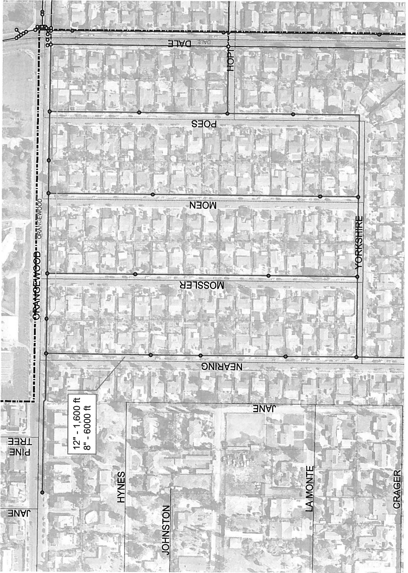
Small Diameter Upsize: Orangewood Dr and Dale St Water Replacement Project
